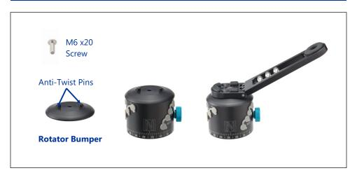
Rotator D6/D8/D12/D16 has central M6 socket and anti-twisting sockets for attaching a foot plate. However, their large diameter limits the upward tilt of foot plate and also makes them vulnerable to dents and scratched. A Rotator Bumper is needed to protect the rotator and provides the clearance for upward tilt. Alternatively, a Quick Mount Mini Adapter System can be used. See more info at the right.
