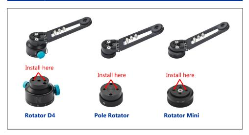
Pole Rotators, Rotator D4 and the Rotator Mini have two M5 sockets separated by 22mm. Foot plate can be attached to them by means of two M5 flat head screws.
